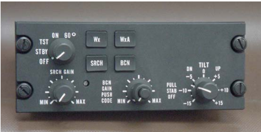
Figure 3.1-1. CP-113K Control Panel
