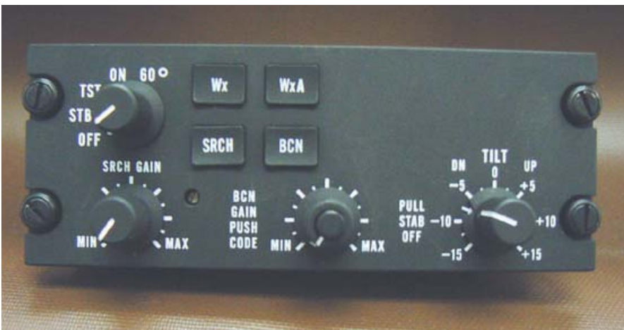
Figure 2.1-3. CP-113K Control Panel
